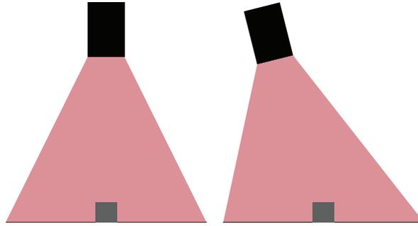
The Swift-E sensor must be mounted no closer than 0.5 m (1.64 ft) to the target objects. The maximum operating range is 6 m (19.68 ft), however at longer operating ranges [greater than 3 m (9.84 ft)], quality of measurement can reduce.
