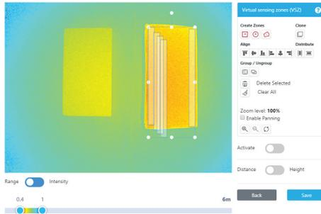
Figure 37 - After Top Alignment and Horizontal Distribution
