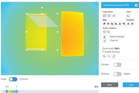
Figure 39 - After Left Alignment And Vertical Distribution
