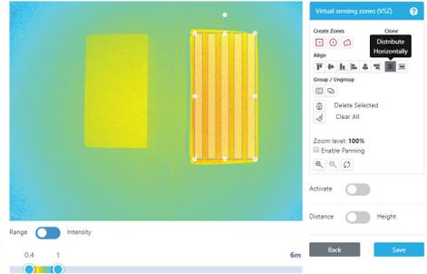
Figure 38 - A Square Sensor - Created, Resized, And Cloned
