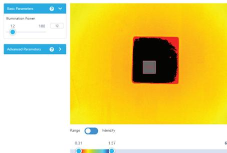
Figure 46 - VSZ is Not Saturated, Measurement is OK
